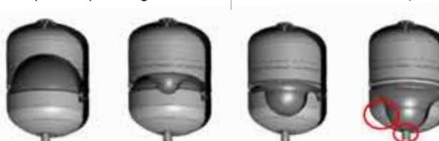
The rubber stretches until it blocks the water inlet/outlet before adhering fully to the inner walls of the vessel, retaining 20% of the usable volume of water inside the vessel.
